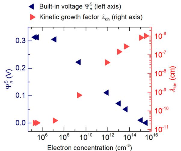
FIG. 2. Electron concentration dependence of the built-in voltage  $\Psi_n^S$  (left axis) and the kinetic growth factor  $\lambda_{\text{kin}}$  (right axis). Values of  $\Phi_{\text{Bn}} = 0.59$  V,  $[\text{B}] = 4.1 \times 10^{15} \text{ cm}^{-3}$ ,  $T = 300$  K, and  $r_n = 1$  nm were used.
