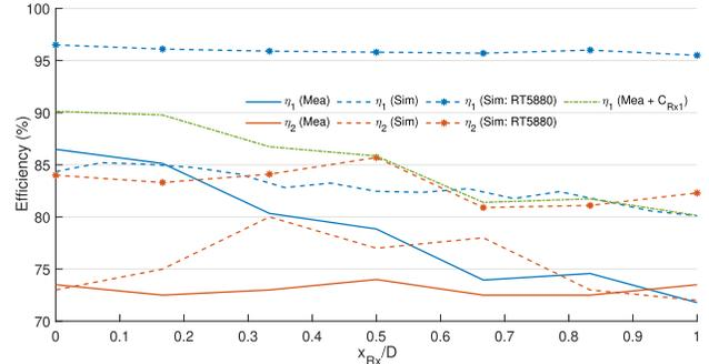
Fig. 15. Efficiency of the proposed system (experimental and numerical results) at frequencies  $f_1$  (denoted as  $\eta_1$ ) and  $f_2$  ( $\eta_2$ ) versus the relative position of the corresponding Rx. Curve for  $\eta_1$  marked “Mea +  $C_{Rx1}$ ” corresponds to the theoretically added matching circuit with the optimal shunt capacitor.
