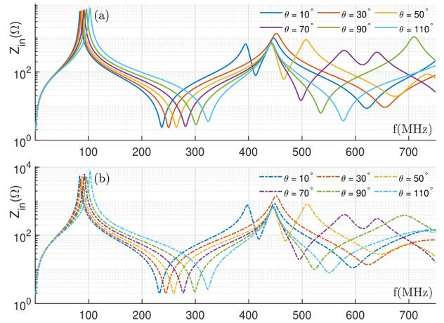
Fig. 7. Absolute value of the input impedance of the HIC with two slits in the effective shield. One slit is fixed at  $\theta_1 = -30^\circ$  and the other slit location angle runs over the following values:  $\theta_2 = 10^\circ, 30^\circ, 50^\circ, 70^\circ, 90^\circ, 110^\circ$ . (a) Circuit model. (b) Full-wave simulation.
