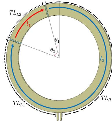
Fig. 5. Proposed HIC with two identical but arbitrarily located slits in the outer strips.  $L_1$  and  $L_2$  represent different parts of the outer strips engendering the lag loads.  $TL_R$ ,  $TL_{L1}$ , and  $TL_{L2}$  represent TLs created by the central metal and inner surface of the outer strips.
