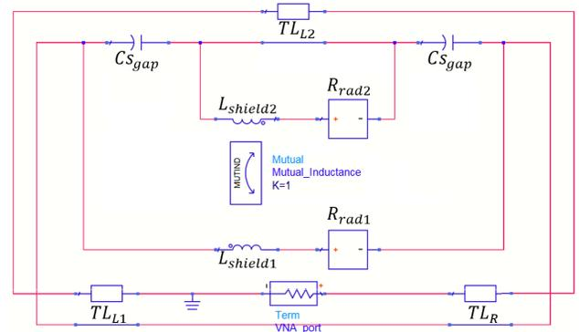
Fig. 6. Circuit model corresponding to dual-slit HICs. The MUTIND module represents the integral coupling between  $L_{\text{shield}1}$  and  $L_{\text{shield}2}$ .
