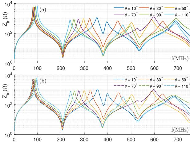
Fig. 4. Absolute value of the input impedance of the HIC with one asymmetrically located slit in the effective shield (outer strips). The angle of the slit runs over the following values:  $\theta = 10^\circ, 30^\circ, 50^\circ, 70^\circ, 90^\circ, 110^\circ$ . (a) Circuit model. (b) Full-wave simulation.
