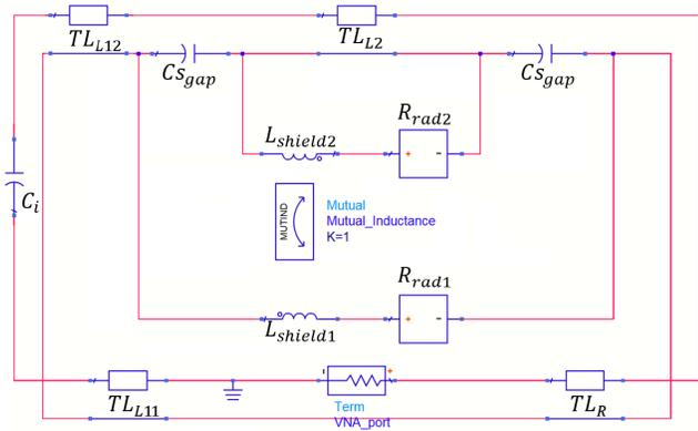
Fig. 8. Circuit model corresponding to HICs with two slits in the outer strips and one slit in the central metal strip between the feeding point  $\theta = \pi$  and  $\theta_2$ .
