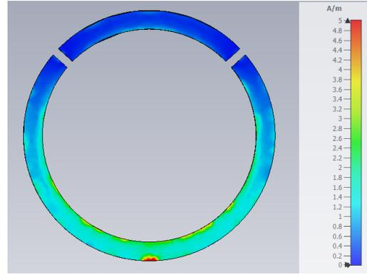
Fig. 9. Current distribution over the outer surface of the effective shield at the second resonance.
