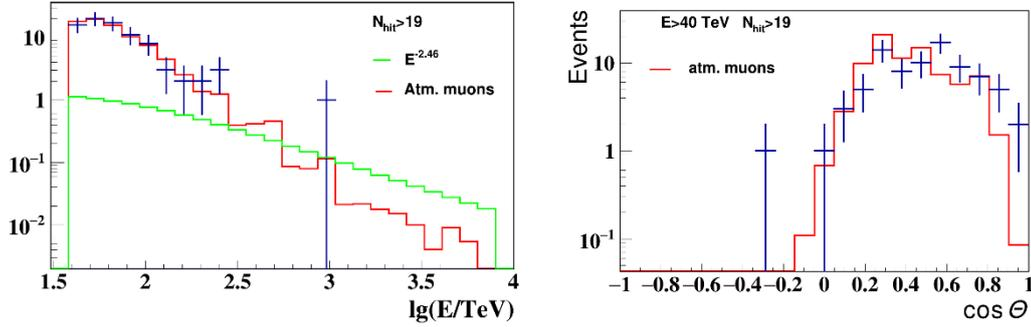
**Figure 3.** *Left:* Energy distribution of data events with  $N_{\text{hit}} > 19$  and  $E > 40$  TeV. Also shown are expected distributions of background events from atmospheric muons (red histograms) and from astrophysical neutrino flux with  $E^{-2.46}$  spectrum (green histogram). *Right:* Cosine of zenith angle distribution of data events with  $N_{\text{hit}} > 19$  and  $E > 40$  TeV and expected distribution from atmospheric muons (red histograms).
