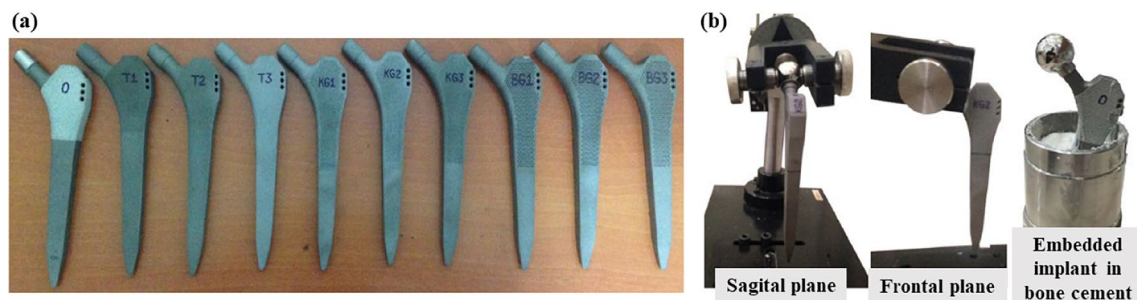
Fig. 28 All specimens produced (a) and experimental setup (b) (images reproduced with permission from reference [246])
