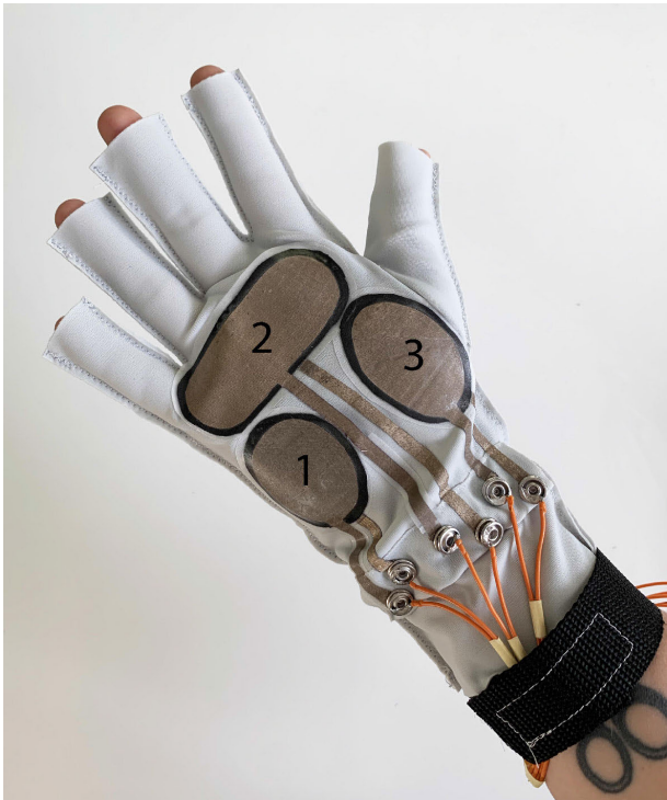
FIGURE 6. Final prototype of pressure sensing glove for right hand.
