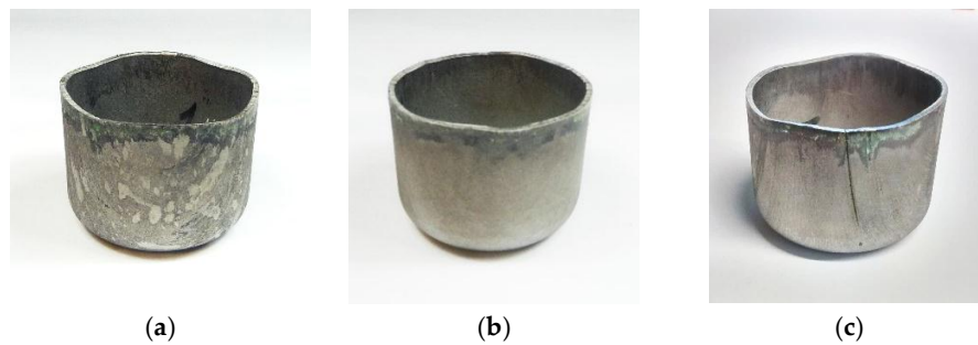
Figure 3. Deep-drawn cups at DR 2.0: (a) steel A; (b) steel B; and (c) steel C.
