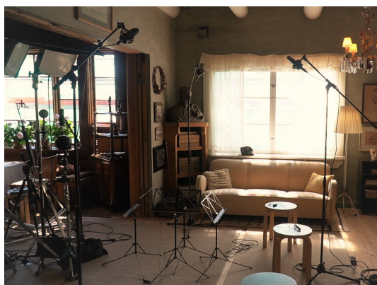
(b) Part of the setup as seen from the piano room. Setup with the camera on the left and microphone arrays behind it. Spot microphones for the three musicians that are in front of the camera.
