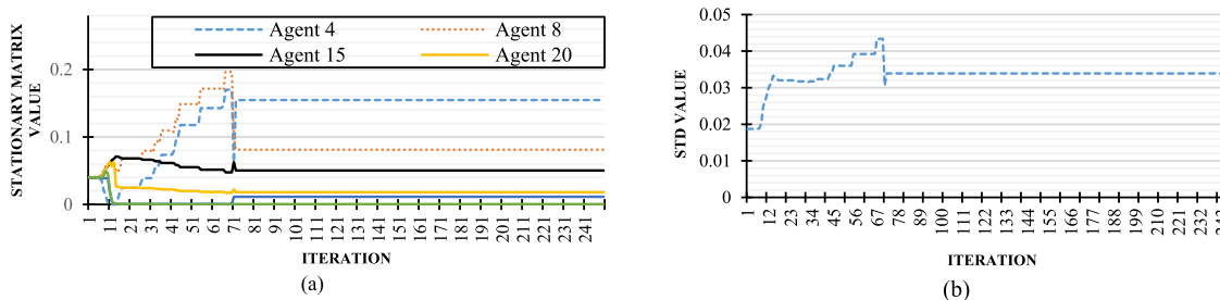
Fig. 18. Simulation results when agent 4 sends fraudulent data to agent 8, with a central entity to supervise convergence problems. (a) Evolution of the stationary distribution matrix. (b) Evolution of the standard deviation value during the iterations.
