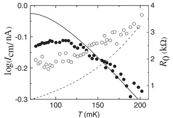
FIG. 3. Temperature dependence of  $I_{cm}$  (●) and  $R_0$  (○) measured at  $V_g = 3.489$  V. The solid curve is a fit obtained from Eqs. (2) and (3) using  $D = 2.2 \times 10^{-3} \text{ m}^2/\text{s}$ ,  $L = 0.4 \mu\text{m}$ , and  $R_n = 17 \text{ k}\Omega$ . The dashed line displays  $R_0$  calculated from Eq. (1) using  $Z_{env} = 400 \Omega$  and  $E_J(T)$  from the above  $T$ -dependence fit.
