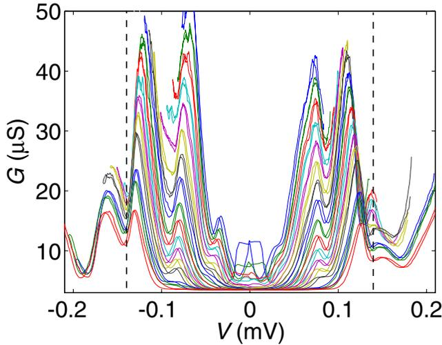
FIG. 4 (color online). Conductance  $G$  vs bias voltage  $V$ . Gate voltage  $V_g$  has been stepped over  $V_g = 3.323 \dots 3.355$  V in steps of 2 mV. The dashed vertical lines indicate locations for the first Andreev reflection process if governed by unrenormalized  $\Delta_{\text{lead}}/e = 139 \mu\text{eV}$ .
