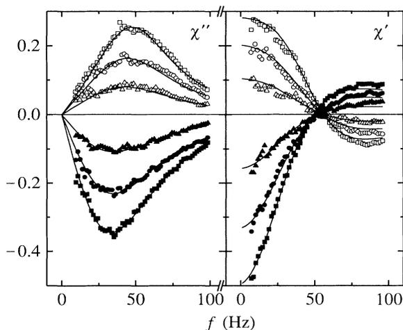
FIG. 1. NMR absorption  $\chi''$  and dispersion  $\chi'$  curves of rhodium nuclei measured in zero magnetic field at initial polarizations  $p = 0.51$  ( $\square$ ),  $0.32$  ( $\circ$ ), and  $0.15$  ( $\triangle$ ) for  $T > 0$ , and  $p = -0.51$  ( $\blacksquare$ ),  $-0.35$  ( $\bullet$ ), and  $-0.17$  ( $\blacktriangle$ ) for  $T < 0$ . The solid lines are least-squares fits of Lorentzian line shapes applied for the absorption and dispersion curves simultaneously (see text).
