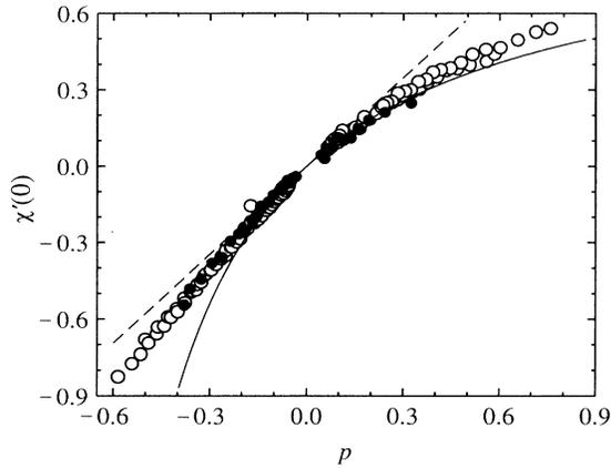
FIG. 2. Static susceptibility  $\chi'(0)$  vs polarization  $p$  of rhodium nuclear spins measured in zero field for our first ( $\bullet$ ) and second ( $\circ$ ) samples. The dashed line is the Curie susceptibility  $\chi_0 = 1.16p$  and the solid curve depicts the mean-field behavior  $\chi = \chi_0/[1 - \chi_0(R + L - D_z)]$ , with  $R = -1.35$ .
