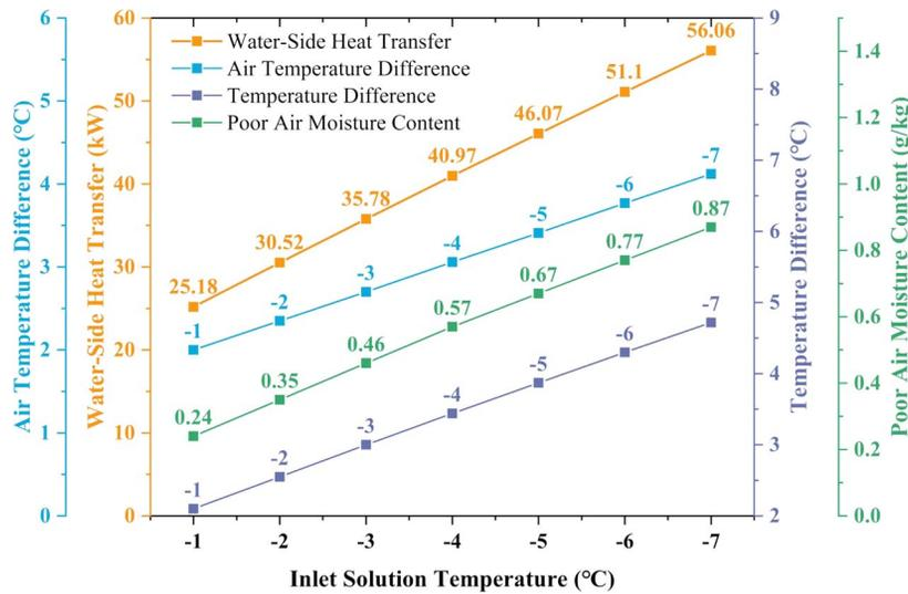
Figure 11. Effect of inlet glycol solution temperature on the performance of heat source towers in winter.
