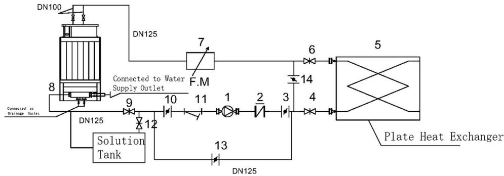
**Figure 1.** Heat source tower heat pump system diagram. (1. Inverter pump; 2. Check valve; 3. Butterfly valve; 4. Electronic valve; 5. Plate heat exchanger; 6. Electronic valve; 7. Test instrument; 8. Heat source tower; 9. Electronic valve; 10. Butterfly valve; 11. Purifier; 12. Electronic valve; 13. Butterfly valve; 14. Butterfly valve.)
