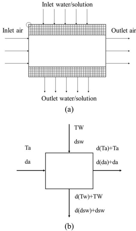
Figure 4. Cross-flow packed heat source tower model.
