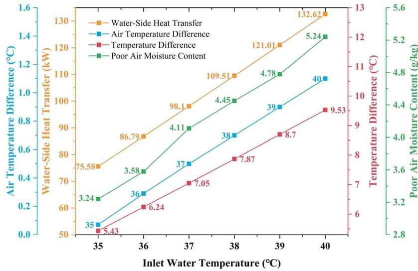
Figure 6. Effect of inlet water temperature on the performance of heat source towers in summer.
