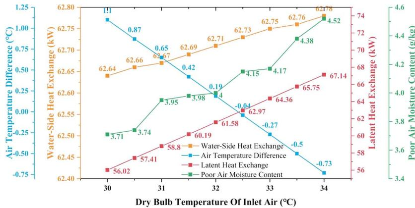
Figure 9. Effect of inlet air dry-bulb temperature on the performance of heat source towers in summer.
