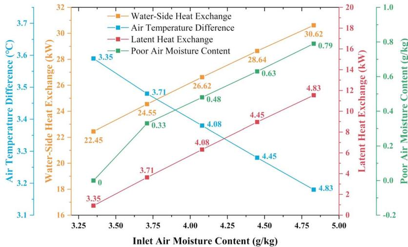
Figure 15. Effect of humidity content of inlet air on the performance of heat source towers in winter.
