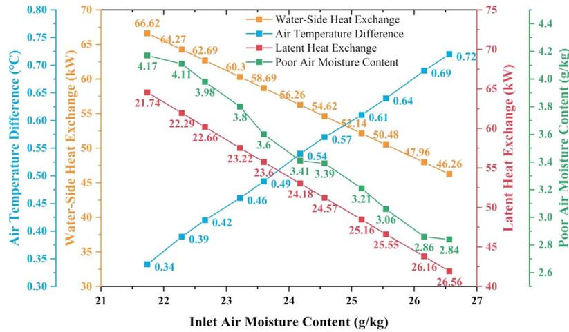
Figure 10. Effect of humidity content of inlet air on the performance of heat source towers in summer.
