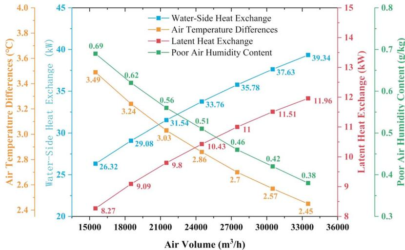
Figure 12. Effect of airflow on the performance of heat source towers in winter.
