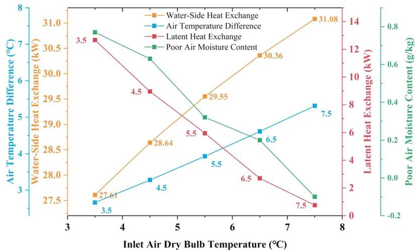
Figure 14. Effect of inlet air dry-bulb temperature on the performance of heat source towers in winter.
