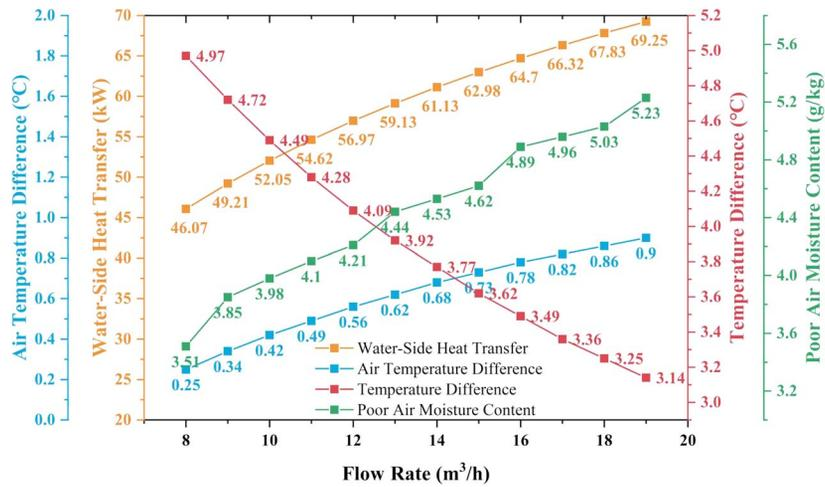
Figure 8. Effect of water flow rate on the performance of heat source towers in summer.
