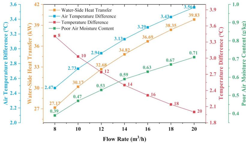
Figure 13. Effect of glycol solution flow rate on the performance of a heat source tower in winter.
