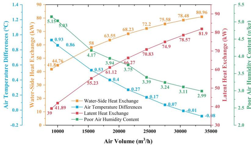
Figure 7. Effect of airflow on the performance of heat source towers in summer.
