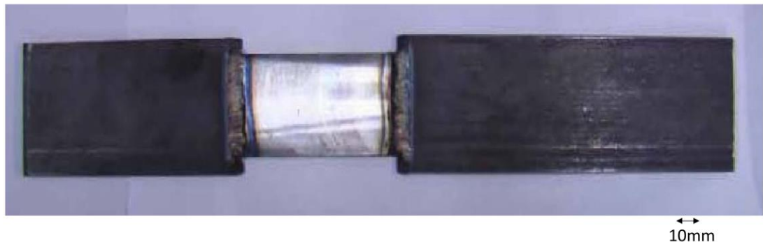
153 154 155 156 157 158 Fig. 1 Longi-Varestraint test specimen with carbon steel support strips welded to each end.
