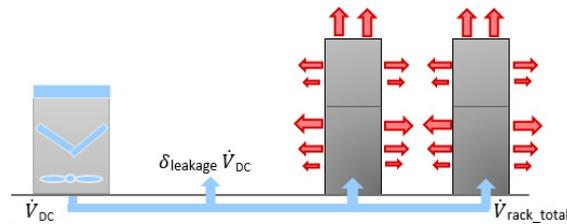
Fig. 3. Air supply with vertical placed server rack.
