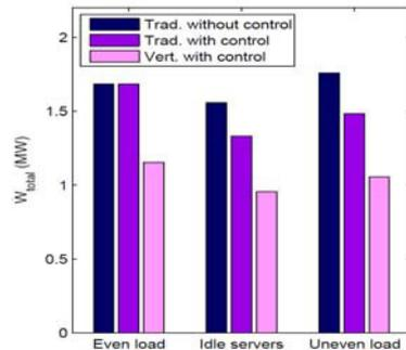
Fig. 5. Total cooling power consumption for all scenarios.
