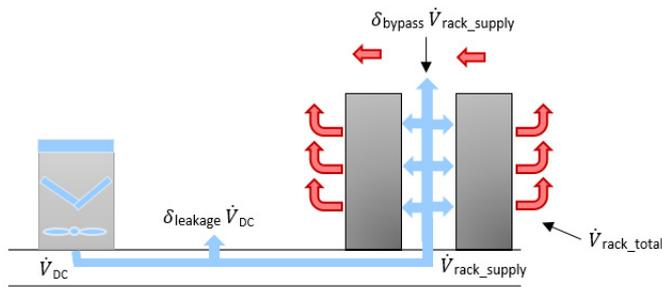
Fig. 2. Traditional hot aisle/cold aisle air supply.
