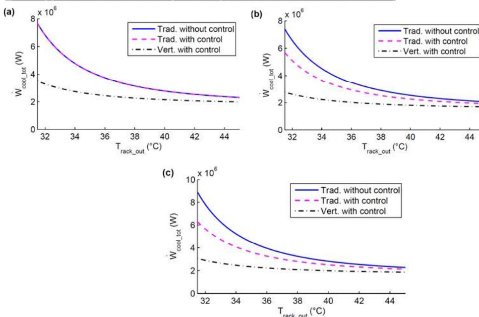
Fig. 4. Total cooling power consumption as a function of the rack outlet temperature for traditional air supply, distributed air flow control and distributed air flow control with vertical placed server; (a) Even load, (b) Idle servers, (c) Uneven load
