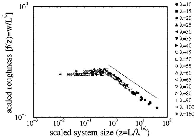
FIG. 3. The scaling function  $f(z) = w/L^\zeta$  of the roughness  $w(L, \lambda)$  vs scaling parameter  $z = L/\lambda^{1/\zeta}$ , where  $\zeta = \zeta_{\text{DP}} = \frac{2}{3}$  for the same data as in Fig. 2. The solid line has a slope of  $\zeta_{\text{RW}} - \zeta_{\text{DP}} = -1/6$ .
