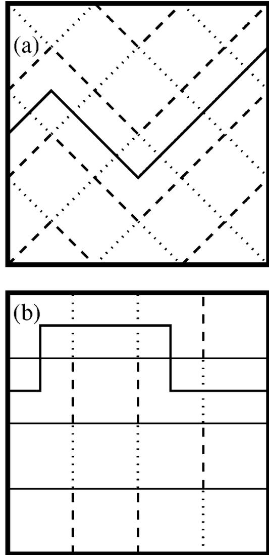
FIG. 1. An example of interface in a random substrate problem, with period  $\lambda=2$ : (a) in  $\{11\}$  orientation; (b) the  $\{10\}$  orientation. The dotted line describes the lower energy bond of the two bonds (in the system of period 2), while the dashed line describes the higher energy bond. A minimum energy path through each system is indicated with a thick solid line.
