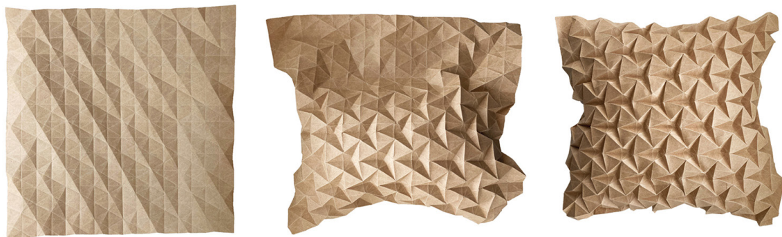
Figure 3. The “framing” process involved in folding a technical origami structure: grid, pre-crease, and collapse. Structures and photos: Laureen Mahler.
