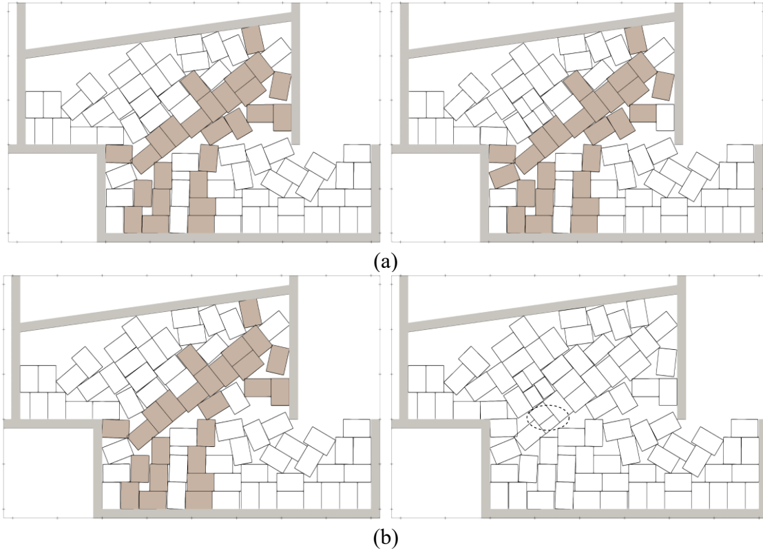
Figure 3: Snapshots from the simulations comparing force chain formation. Left column shows figures from a simulation without the breakage model while those in the right column are from a simulation with the breakage model. Force chain is (a) first forming near the shear plane in both simulations, and then (b) force chain in the simulation with the breakage model collapses due to block breakage.
