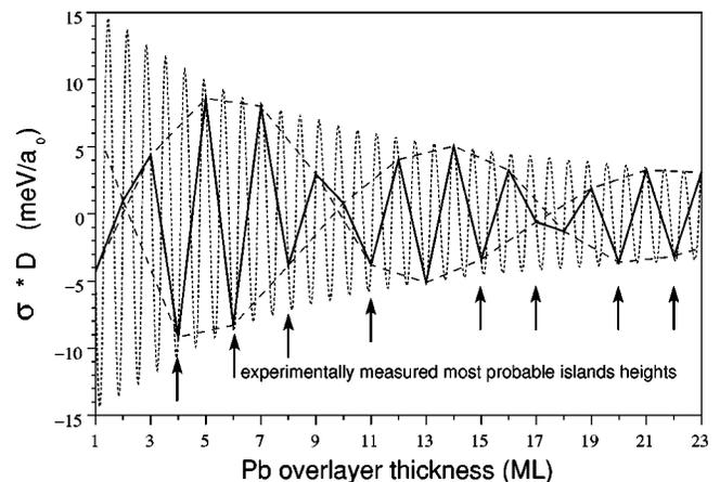
FIG. 3. Oscillating part of the total-energy per surface area of Pb/Cu(111) system ( $\sigma$ ) multiplied by the Pb slab thickness  $D$ . The dotted line is a function of the continuous Pb-SJ thickness. The solid line connects the values corresponding to completed ML’s. The dashed lines guide the eye in order to show the supershell structure. The arrows denote the measured thicknesses of the most abundant island heights (Ref. 5).
