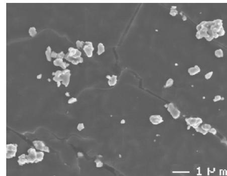
FIG. 2. Scanning electron microscope image of TiO<sub>2</sub> powder.
