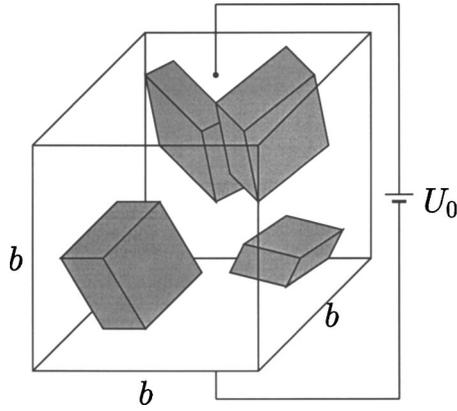
FIG. 6. Illustration of the computation domain. Inclusions with permittivity  $\epsilon_i=114$  ( $\text{TiO}_2$ ) were placed randomly into an environment with permittivity  $\epsilon_e=3.7$  (epoxy), and a static electric field was applied. The boundary conditions were PEC and PMC, corresponding to an ideal capacitor.
