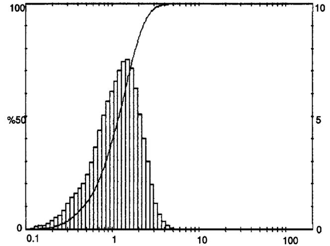
FIG. 1. Particle size distribution of TiO<sub>2</sub> powder in micrometers.
