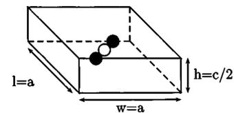
FIG. 8. The smallest cell, which contains a titanium atom and two oxygen atoms.
