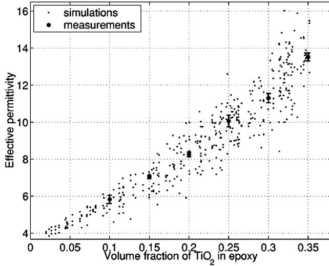
FIG. 9. Modeled (dots) and measured (asterisks) effective permittivities for TiO<sub>2</sub>/epoxy composite. The deviations of the measured permittivities were calculated using Eq. (2). In the simulations, the field solution for each Monte Carlo sample was calculated three times, corresponding to the three orthogonal field excitations. Accordingly, for every volume fraction, permittivities of  $\epsilon_x$ ,  $\epsilon_y$ , and  $\epsilon_z$  are presented.
