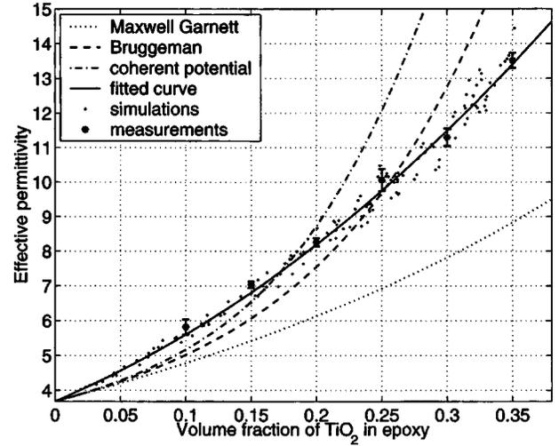
FIG. 10. Modeled (dots) and measured (asterisks) effective permittivities of TiO<sub>2</sub>/epoxy composite, as in Fig. 9, but now the simulated permittivities are shown averaged over  $\epsilon_x$ ,  $\epsilon_y$ , and  $\epsilon_z$  according to Eq. (6) for every Monte Carlo sample. Equation (9) was fitted to the simulations and is marked with a solid line.
