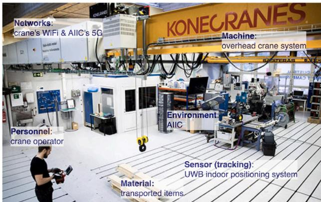
Fig. 6. Overview of the physical space for the case study of in-plant material flow tracking: The physical space at the AIIC involves transported materials, an overhead crane system, a UWB indoor positioning system, and a human operator managing the process within AIIC's network environment.
