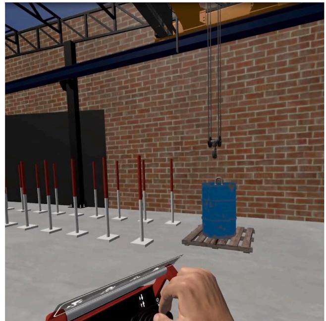
Fig. 9. A scene captured from our VR application for remote crane operation and material flow tracking: Users can remotely monitor material flows and control the crane through a virtual representation of the physical crane operating space with VR headsets.
