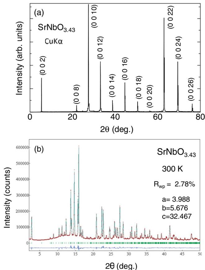
FIG. 2. (Color online) (a) X-ray diffraction pattern along the  $c$  axis and (b) synchrotron powder x-ray diffraction pattern of a ground single crystal.
