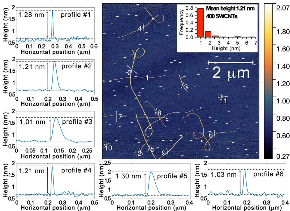
FIG. 4. AFM characterization of SWCNTs synthesized at 880 °C with  $N \approx 10^5 \text{ cm}^{-3}$ . The scan window size is  $7 \times 7 \mu\text{m}^2$ . The vertical height profiles of the cross sections 1–6 are shown around the scan window, representing heights between 1 and 1.3 nm (profiles 7–12 can be found in Ref. 14). The histogram shows the statistics of 400 height profiles, with the mean at 1.21 nm.
