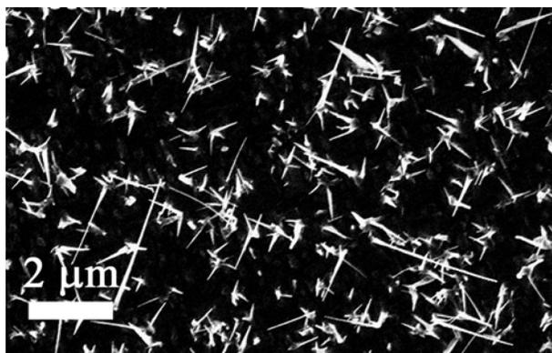
FIG. 1. SEM images of plane view of (Ga,Mn)As NWs arrays.
