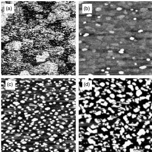
FIG. 1. AFM images of GaAsN layers with thicknesses of (a) 3 ML, (b) 4 ML, (c) 5 ML, and (d) 6 ML deposited on InP at the temperature of 530 °C. The samples were annealed *in situ* at 610 °C for 20 s. The scan size is  $1 \times 1 \mu\text{m}^2$ .
