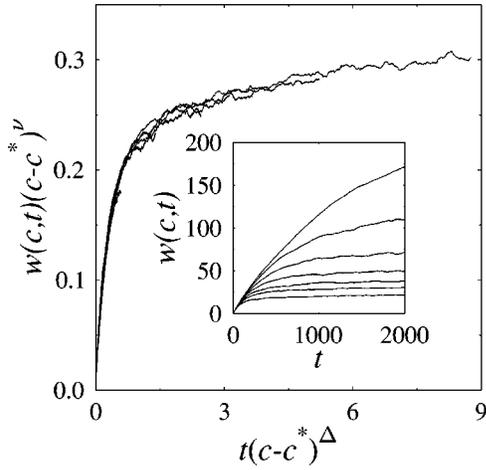
FIG. 4. Crossover scaling function  $f(t/\tau_c)$  of the global width  $w(c,t)$ , as defined in Eq. (6). The unscaled data for different concentrations ( $c=0.594, 0.60, 0.605, 0.61, 0.615, 0.62$ , and  $0.63$ , from top to bottom, and  $L=1000$ ) are shown in the inset. The data collapse has been obtained using  $\nu=1.3$  and  $\Delta=1.65$ . See the text for details.
