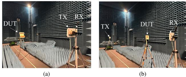
Fig. 7: OTA measurement setup: (a) bistatic collocated configuration, (b) bistatic dislocated configuration.
