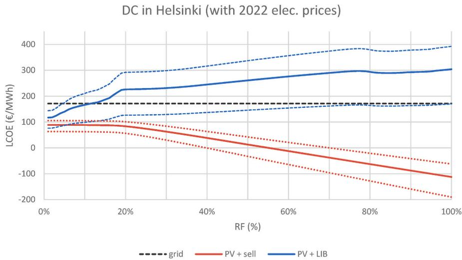
**Fig. 10.** Levelized cost of energy (LCOE) of the modelled PV systems in S1 (Helsinki) as a function of the attained renewable fraction (RF) with year 2022 electricity prices. The dashed lines showcase the sensitivity analysis on solar PV and LIB system costs, according to the lower and upper values presented in Table 2.
