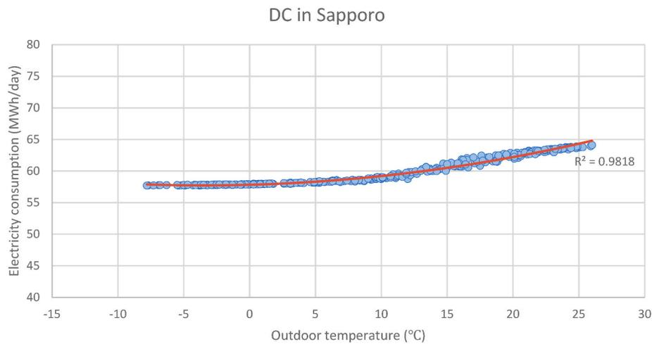
Fig. 8. Correlation between daily electricity consumption and average daily outdoor temperature of the modelled 2.5 MW DC in Sapporo (S3).
