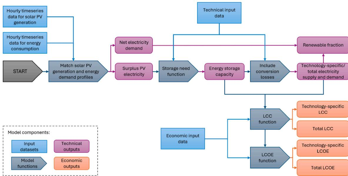
Fig. 2. Inputs, functions, and outputs of the employed MATLAB energy system model.
