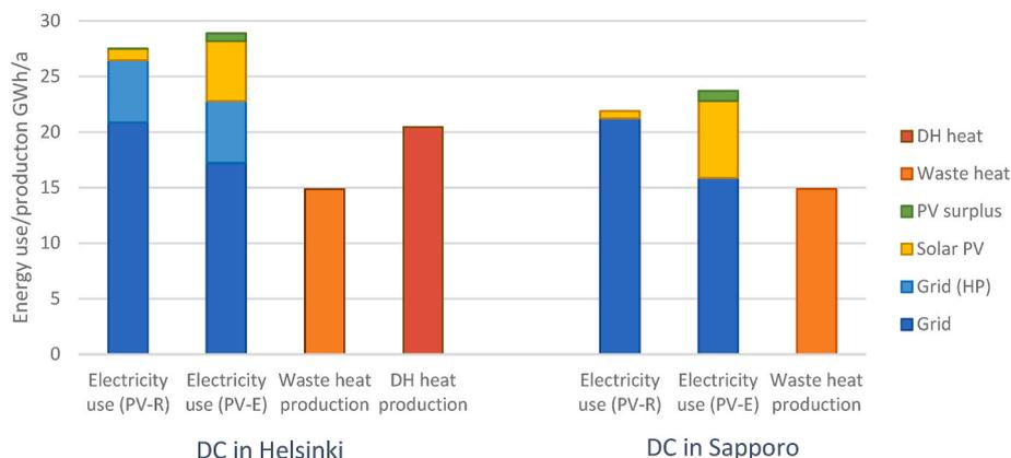
Fig. 4. Electricity use, solar PV electricity surplus, available waste heat, and DH production for the modelled 2.5 MW DCs in Helsinki (S1) and Sapporo (S3).
