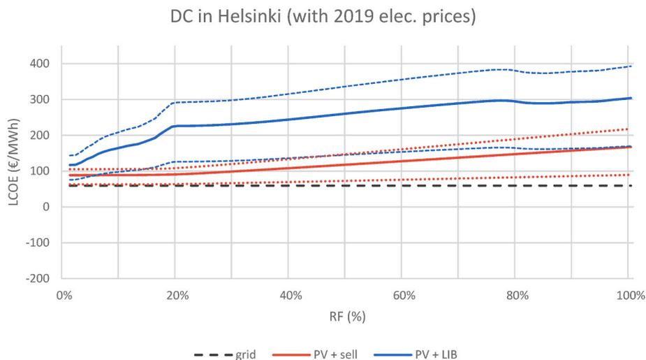
**Fig. 9.** Levelized cost of energy (*LCOE*) of the modelled PV systems in S1 (Helsinki) as a function of the attained renewable fraction (RF) with year 2019 electricity prices. The dashed lines showcase the sensitivity analysis on solar PV and LIB system costs, according to the lower and upper values presented in Table 2.
