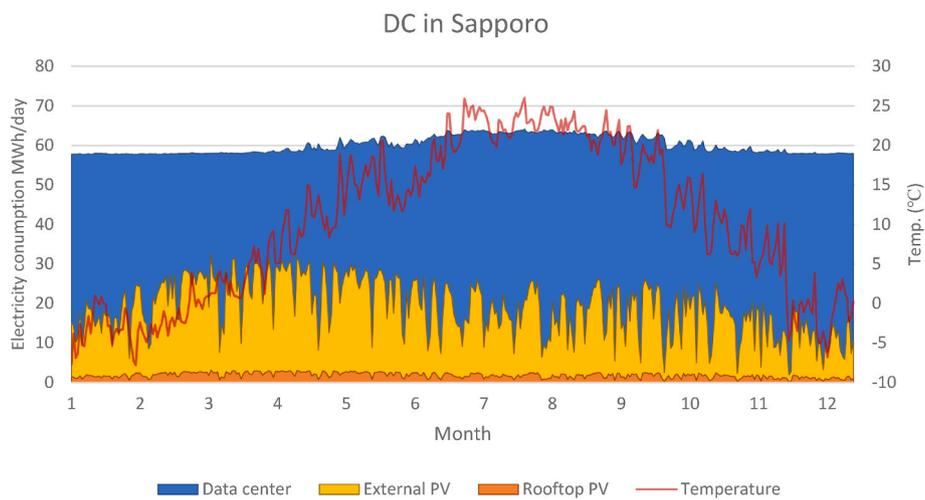
Fig. 6. Daily electricity consumption, solar PV generation, and average outdoor temperature for the modelled 2.5 MW DC in Sapporo (S3). The DC electricity consumption is based on modelled data.
