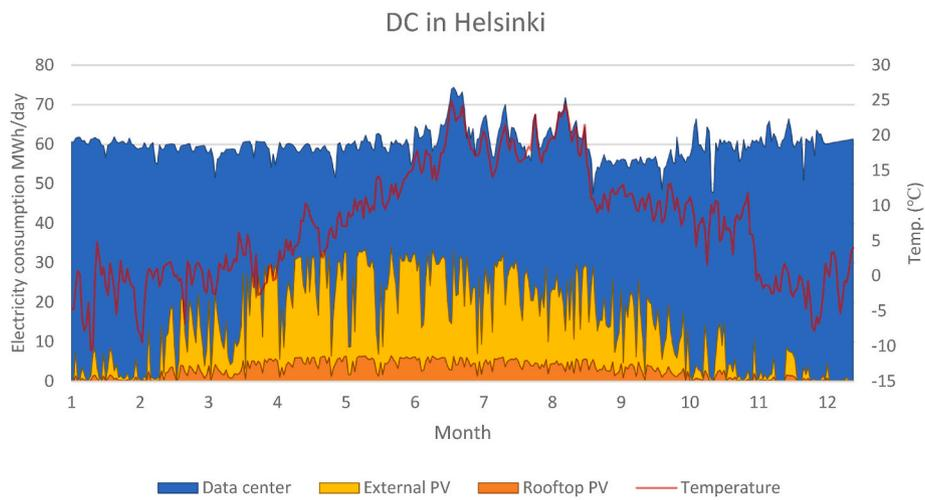
Fig. 5. Daily electricity consumption, solar PV generation, and average outdoor temperature for the modelled 2.5 MW DC in Helsinki (S1). The DC electricity consumption is based on historical data.
