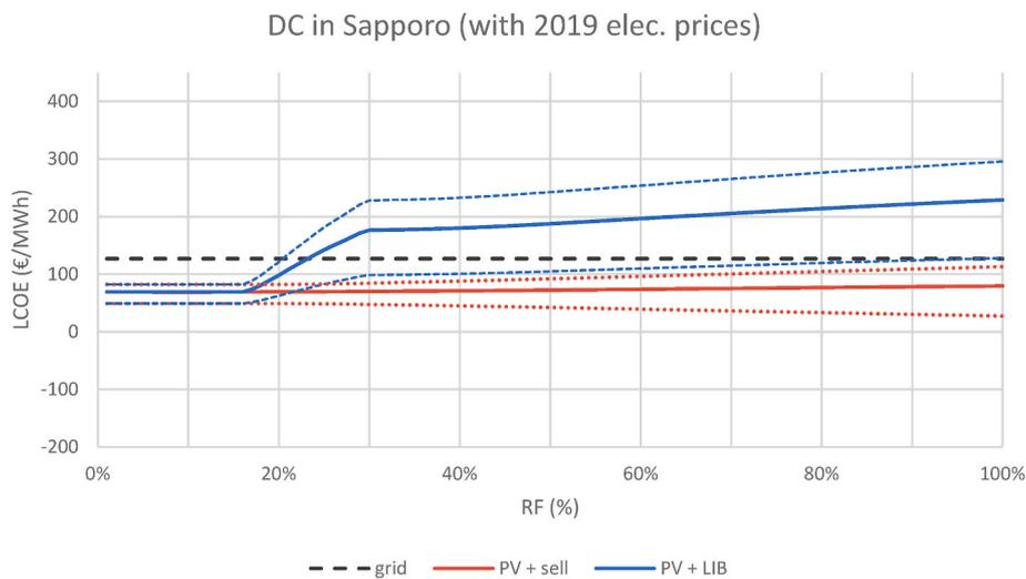
**Fig. 11.** Levelized cost of energy (LCOE) of the modelled PV systems in S3 (Sapporo) as a function of the attained renewable fraction (RF) with year 2019 electricity prices. The dashed lines showcase the sensitivity analysis on solar PV and LIB system costs, according to the lower and upper values presented in Table 2.
