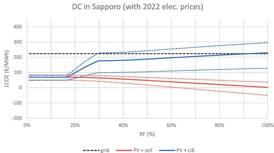
**Fig. 12.** Levelized cost of energy (LCOE) of the modelled PV systems in S3 (Sapporo) as a function of the attained renewable fraction (RF) with year 2022 electricity prices. The dashed lines showcase the sensitivity analysis on solar PV and LIB system costs, according to the lower and upper values presented in Table 2.
