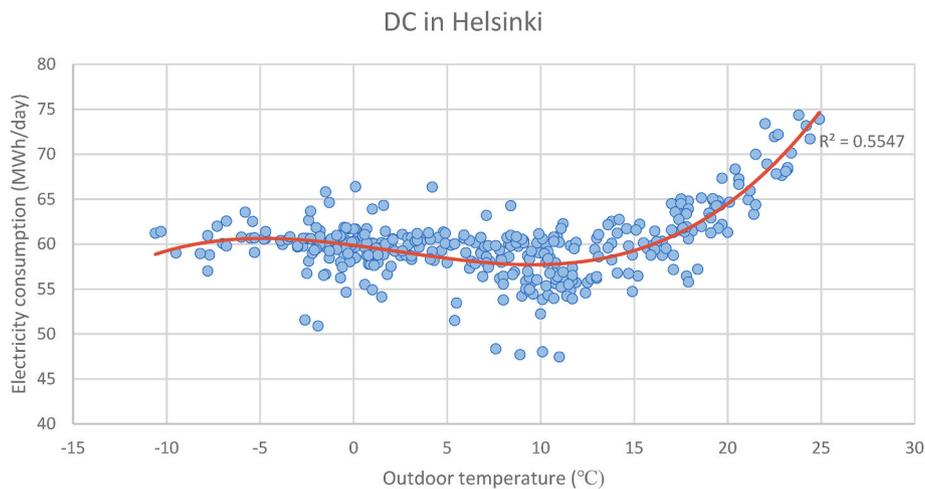
Fig. 7. Correlation between daily electricity consumption and average daily outdoor temperature of the modelled 2.5 MW DC in Helsinki (S1).
