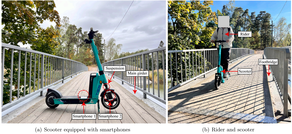
Fig. 11. Scooter, rider, and smartphones in field tests.
