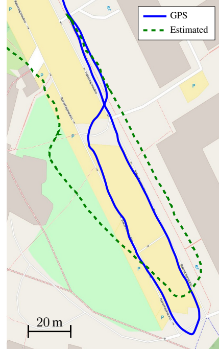
Fig. 2. Estimated trajectory (green, dashed) together with the GPS reference path (blue, solid), overlaid onto the local map 3 .
