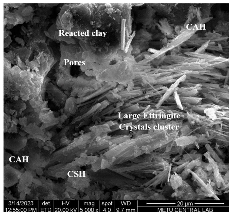
**Figure 10.** SEM photo of treated sample, which includes major structures.
