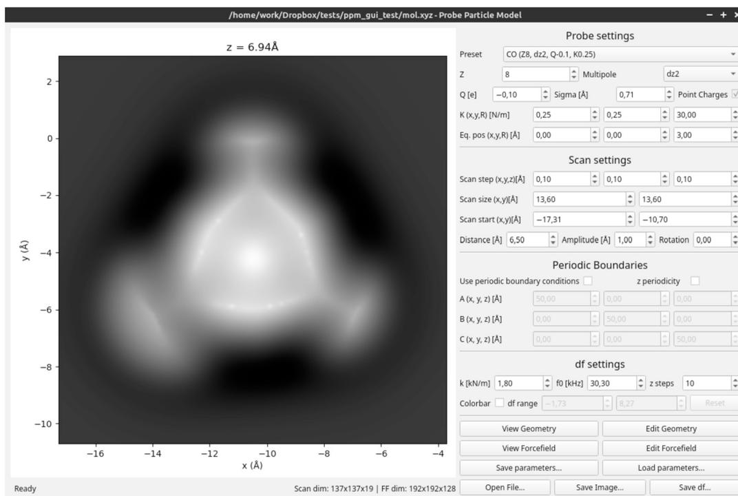
**Fig. 6.** Interactive GUI for GPU-accelerated `ppa_fm` simulations. The user can interactively modify imaging parameters by using input boxes or a mouse-wheel, and image contrast is updated automatically.
