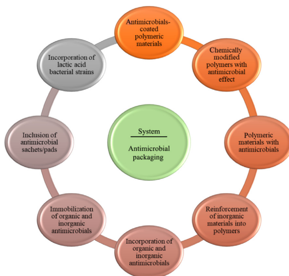
Fig. 13. System development of active packaging using antimicrobial agents by different methods (Kanmani and Rhim, 2014).
