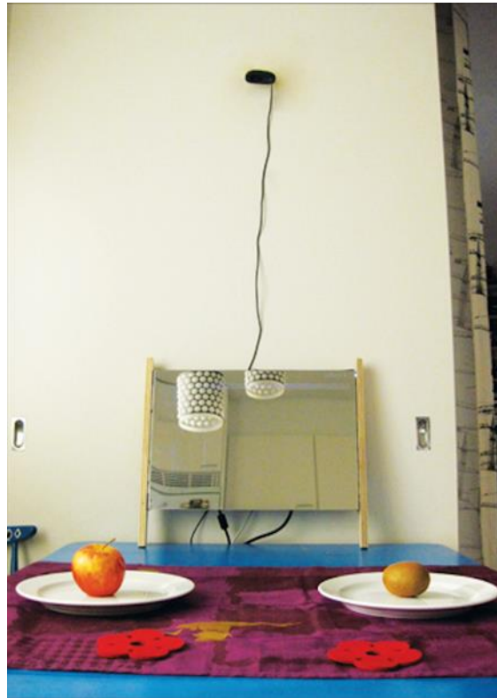
Figure 5. MealWeaver-setup in a test situation, using a webcam as the input, and the semi-transparent mirror as the output.
