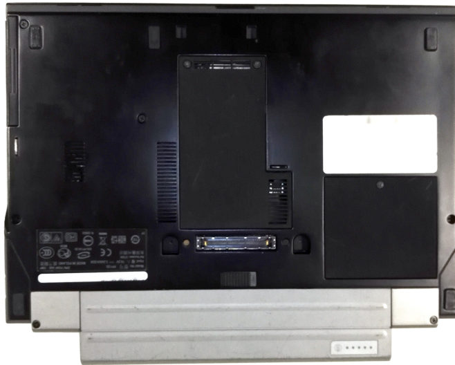
Figure 6. Laser sintered plastic cover (middle) attached to a Dell Latitude 4300 portable computer.
