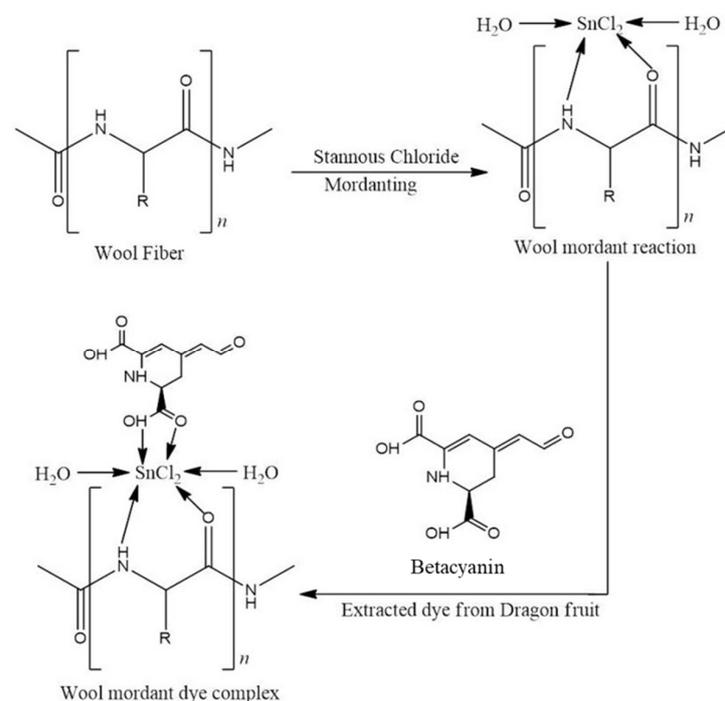
**Figure 6.** Complex reaction mechanism of wool–stannous chloride mordant for natural dye extracted from dragon fruit.
