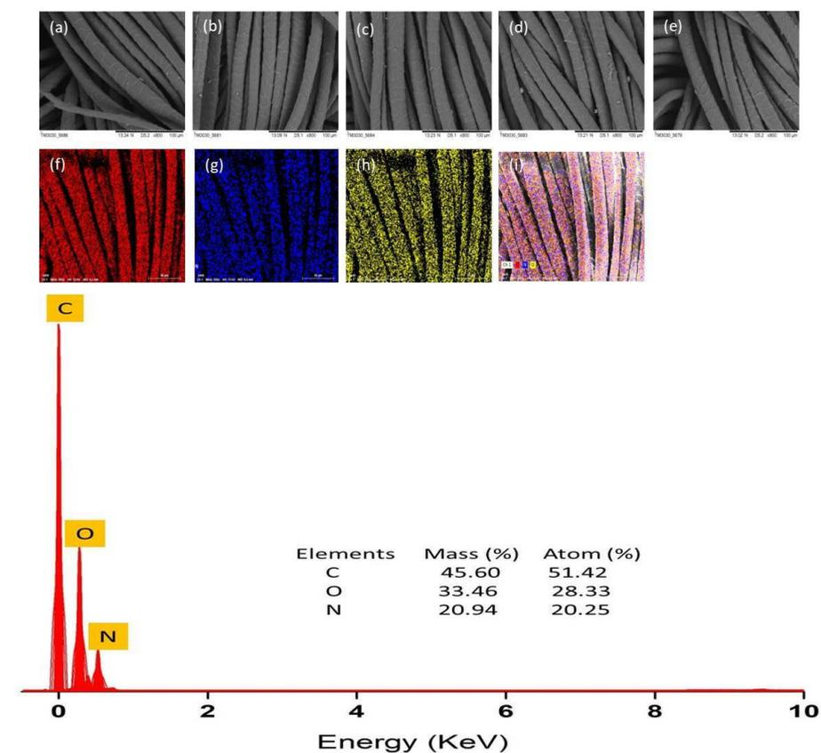
**Figure 2.** SEM, EDX, and mapping images of (a) undyed wool, (b) wool dyed without mordant, and (c–e) wool dyed with different mordant, (f) carbon mapping, (g) nitrogen mapping, (h) oxygen mapping, and (i) mixed mapping.
