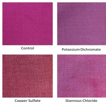
**Figure 1.** Color shades obtained by wool samples after mordanting, dyeing, and control sample.
