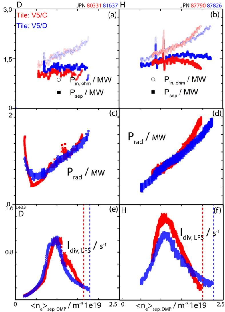
**Fig. 5.** Comparison of experimental input, radiated and separatrix power, and the LFS plate-integrated ion current at different strike point locations in deuterium (a,c,e) and hydrogen (b,d,f) plasmas.
