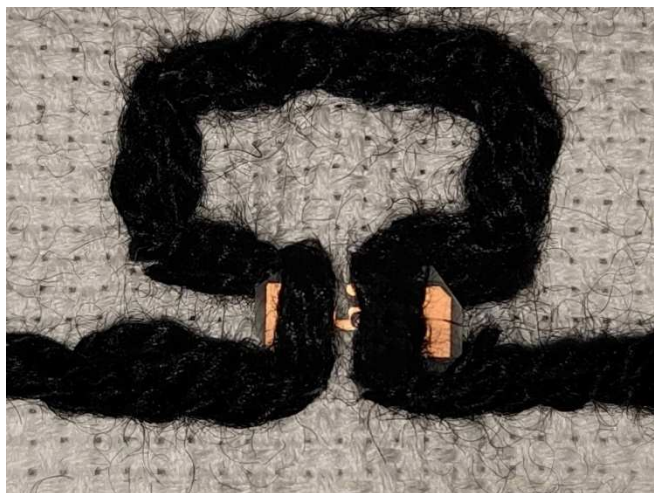
Fig. 1. The studied passive UHF RFID antenna fabricated using polypyrrole yarn and its antenna geometry in millimeters (Top) and the close up of the connection between the antenna and the IC pads (Bottom).
