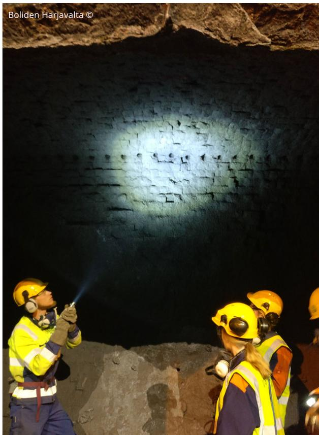
Fig. 2. The inside view of the sampled PSC at Boliden Harjavalta prior to dismantling (Reprinted with permission from Boliden Harjavalta ©).
