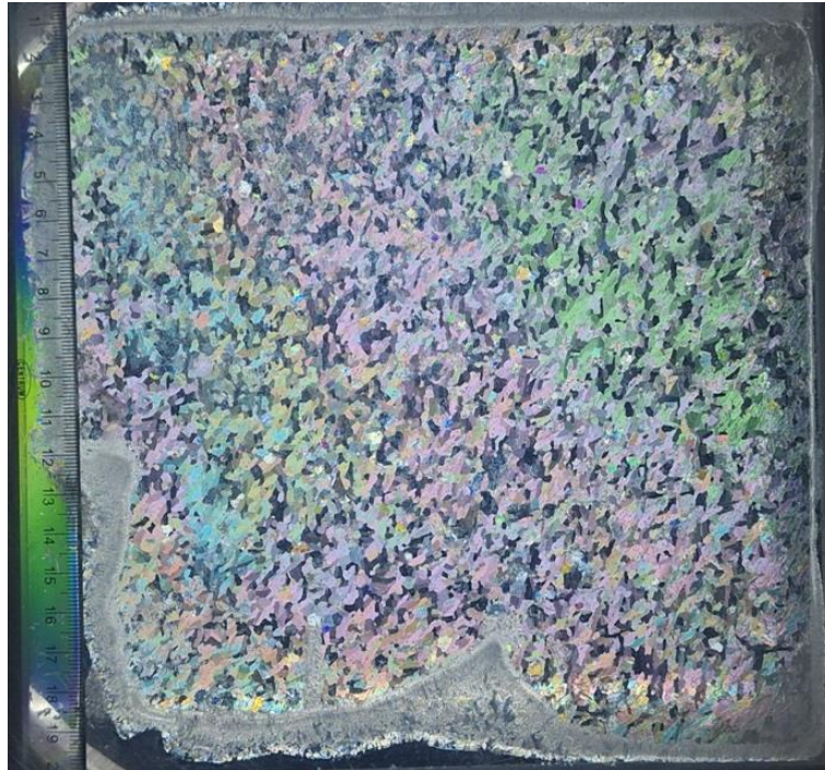
Figure 2. Horizontal 1 mm thin section of the grown ice. Sample is 20 mm from the top.
