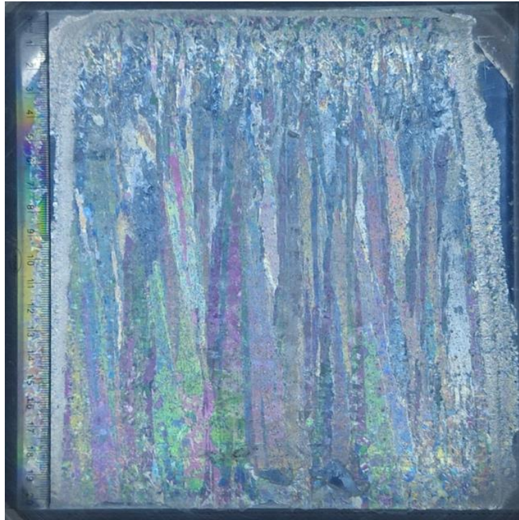
Figure 3. Vertical 1 mm thin section of the grown ice showing the top 200 mm of the ice.
