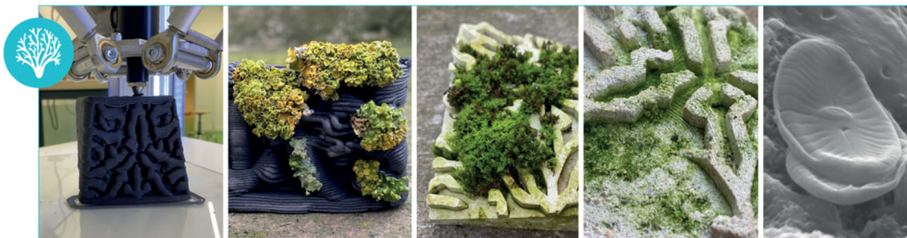
Figure 3. Prototypes, transplants and first signs of spontaneous colonisation on bio-receptive materials.
