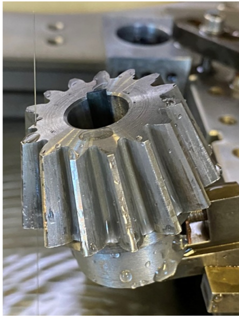
Fig. 12. Replication of TFF with the help of an EDM.
