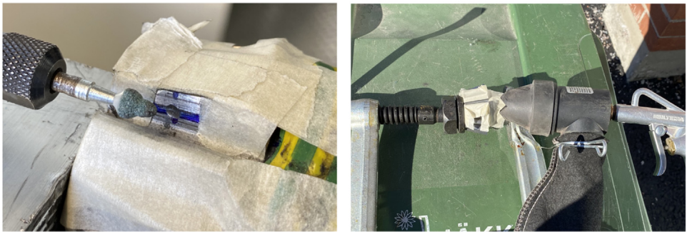
(a) Replication of pitting using abrasive machining.
