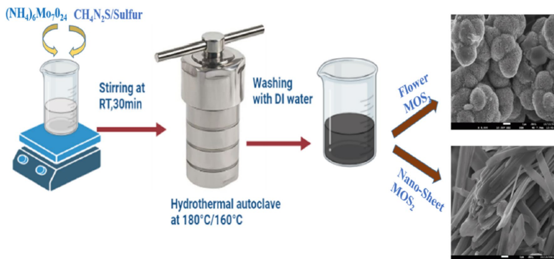
Fig. 6 Diagram showing the hydrothermal synthesis process for creating MoS 2 nanoflowers and nanosheets. Source: [138]
