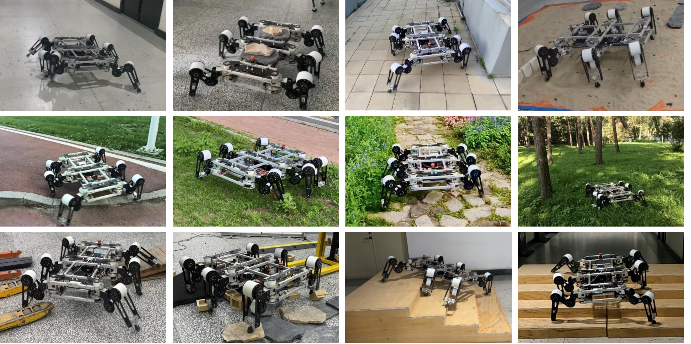
Fig. 2. We tested the performance of the hexapod in a variety of environments, indoor and outdoor, and our method showed good performance. The hexapod robot moves robustly and efficiently with a periodic gait.
