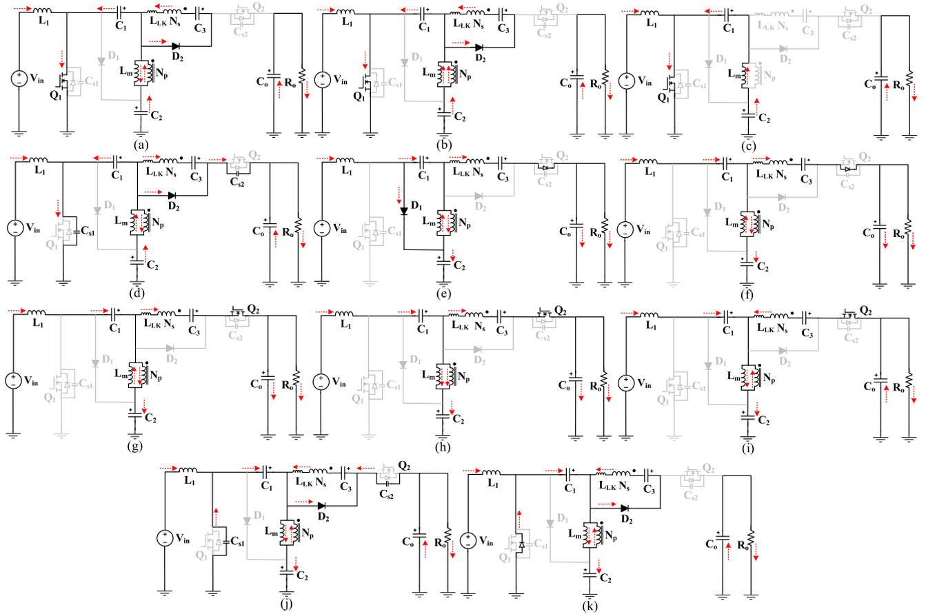
**FIGURE 3.** Operation modes of the proposed converter, (a) mode 1 [ $t_0 - t_1$ ], (b) mode 2 [ $t_1 - t_2$ ], (c) mode 3 [ $t_2 - t_3$ ], (d) mode 4 [ $t_3 - t_4$ ], (e) mode 5 [ $t_4 - t_5$ ], (f) mode 6 [ $t_5 - t_6$ ], (g) mode 7 [ $t_6 - t_7$ ], (h) mode 8 [ $t_7 - t_8$ ], (i) mode 9 [ $t_8 - t_9$ ], (j) mode 10 [ $t_9 - t_{10}$ ], (k) mode 11 [ $t_{10} - t_{11}$ ].
