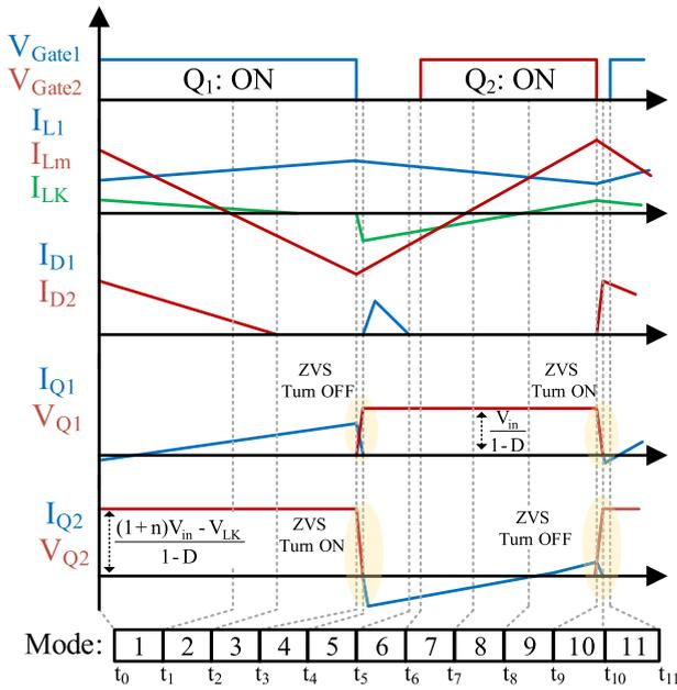
FIGURE 2. Key waveforms.
