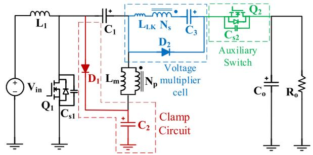
FIGURE 1. The proposed converter.
