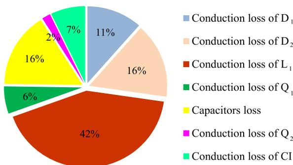
**FIGURE 7. Loss breakdown of the proposed converter for 100 W output power.**
