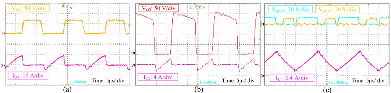
**FIGURE 9.** The experimental waveforms under light load. (a) Voltage and current of  $Q_1$ , (b) Voltage and current of  $Q_2$ , (c) Gate-source voltage of  $Q_1$ , gate-source voltage of  $Q_2$ , and input current.
