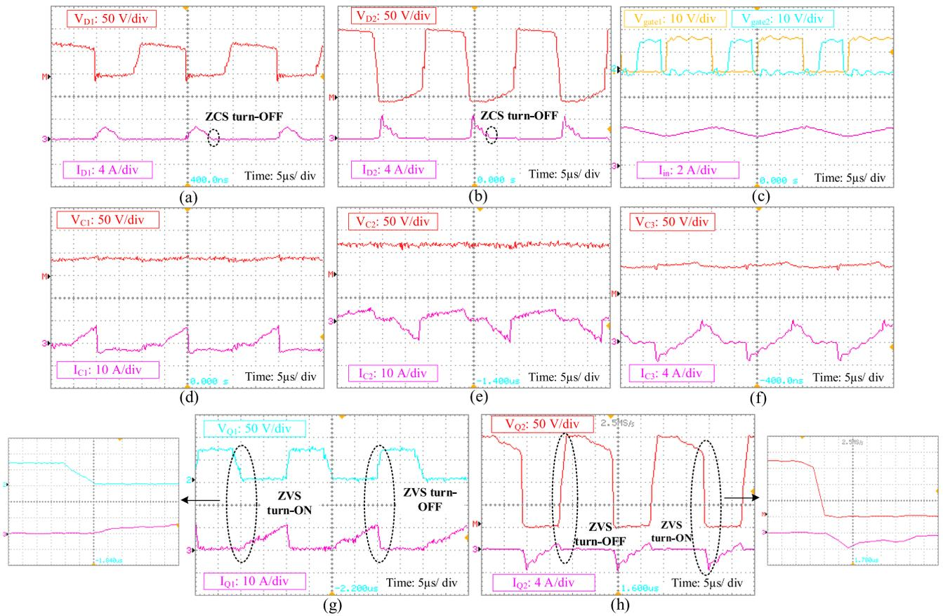
**FIGURE 8.** The experimental waveforms under full load. (a) Voltage and current of  $D_1$ , (b) Voltage and current of  $D_2$ , (c) Gate-source voltage of  $Q_1$ , gate-source voltage of  $Q_2$ , and input current, (d) Voltage and current of  $C_1$ , (e) Voltage and current of  $C_2$ , (f) Voltage and current of  $C_3$ , (g) Voltage and current of  $Q_1$ , (h) Voltage and current of  $Q_2$ .
