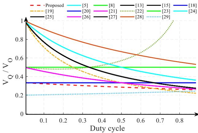
FIGURE 5. The normalized voltage stress across main switches in the investigated topologies.
