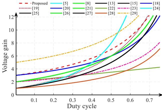
FIGURE 4. Voltage gain for investigated converters.
