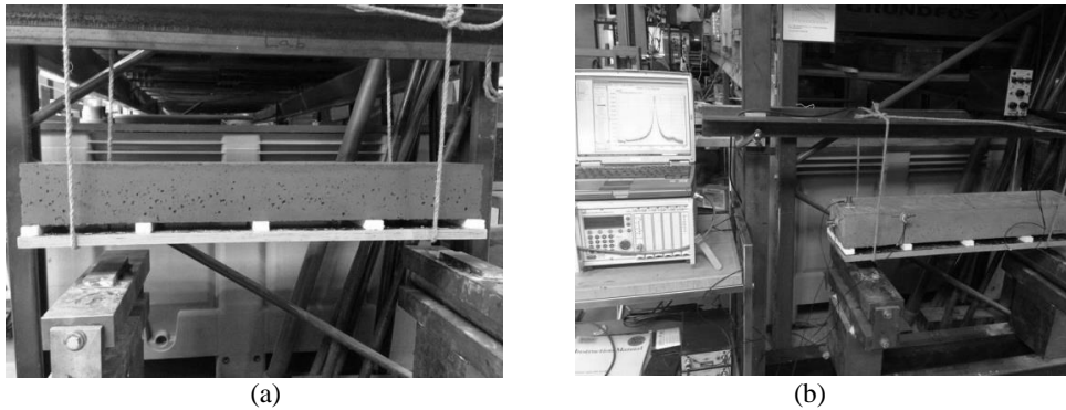
Figure 1 – The suspended beam and the position of the accelerometers.
