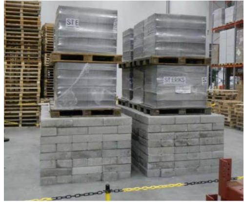
Figure 2 – Loaded area (left) and loads consisting of pallets of concrete pavers (right).
