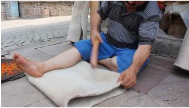
Figure 8: The master re-forms the shape of the felted wool, with the help of his stick, after the first iteration of the machine pressure. Maker: İlyas from the studio. Photography: Author, August, 2017.
