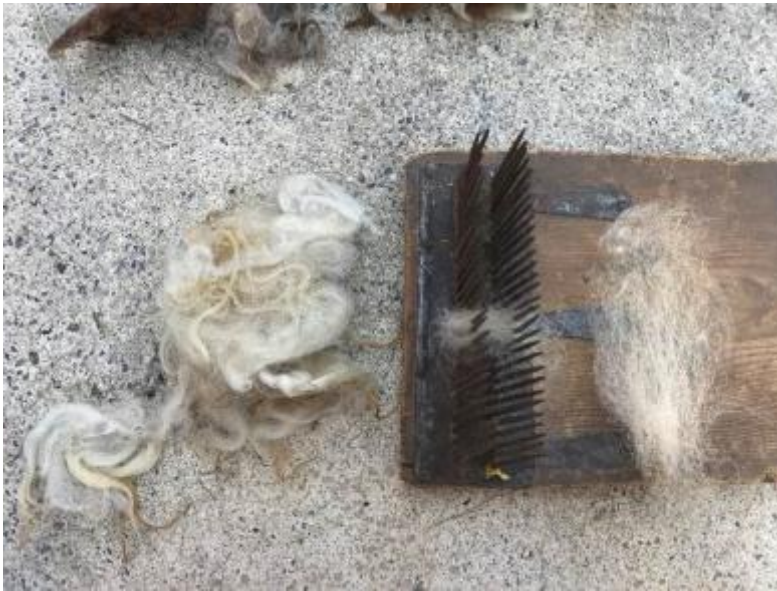
Figure 4: The ancient tool for roving and the wool before (left) and after (right) roving. Photography: Author, July, 2017.
