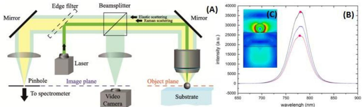
**Figure 3.** (a) A schematic illustration of multifunctional experimental setup for Raman for PL experiments. (b) PL enhancement from perovskite with silicon nanoparticles: maximum signal from perovskite with Si nanoparticles (black line); averaged signal from plain perovskite (red line); averaged signal from perovskite with Si nanoparticles (blue line). (c) Result of numerical calculation of electric fields near a silicon nanoparticle ( $D = 200$  nm). The excitation wavelength is 633 nm.
