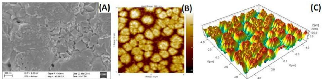
**Figure 1.** (a) SEM image of perovskite surface without nanoparticles. AFM images of perovskite: (b) 2D and (c) 3D view.
