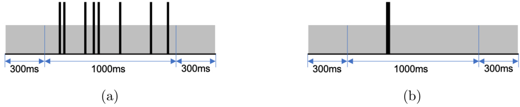
Figure 2: Configuration of target stimuli with the masker. The grey area represents the masker noise, and the short vertical lines represent the target bursts. (a) Stimuli with sets of different burst rates: multiple target bursts, comprising 1-ms single bursts, are randomly distributed within the 300–1300 ms time slot of the masker noise. (b) Stimuli with different burst duration: a single target burst, 1–30 ms in duration, is located in a random temporal position within the 300–1300 ms time slot of the masker noise.
