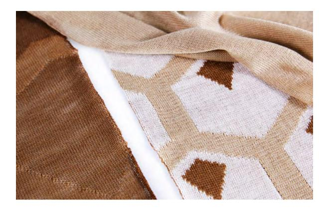
Lignin can find its way into textiles via several routes. Either it is added prior to fibre spinning, or it comes as part of the raw material, such as in recycled cardboard. From the design point of view lignin gives the possibility of communicating the origin of man-made cellulose fibres in a visual and intuitive way [3]. Brown from the birch, or khaki from cardboard could be used as aesthetical eco-statements in design.
