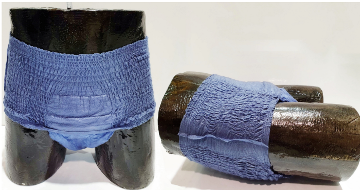
Fig. 4. Measurement setup to analyze the gravitational pull effect with on-torso diapers in both standing and lying positions.
