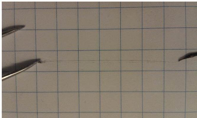
Figure 2 PF11-2.5 monofilament. The square grids are approximately 7x7 mm<sup>2</sup> in dimension
