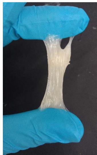
Figure 1 Spinning dope of PAA-16DGE (1:1 ratios, no cellulose or graphene)
